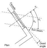
Figure 1 Dead angle and angle of the sun beam incidence  $\Theta_1$
