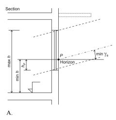
Figure 2 Rule for location of the reference point.
